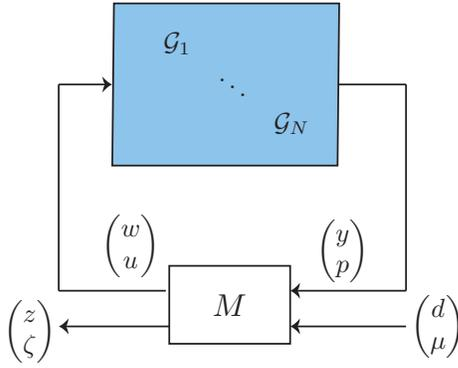
**Figure 1: Interconnected system with hybrid inputs  $(d, \mu)^T$  and hybrid outputs  $(z, \zeta)^T$ .**
