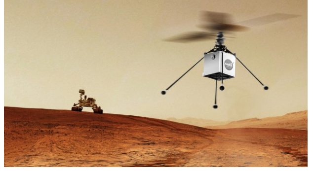
Fig. 1: Artist's rendering of the proposed helicopter to scout for the Mars rover. The helicopter can fly ahead and send information back to the rover about the presence of any obstacles. [1].
